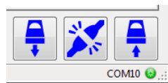
Figure 21 - Action buttons when an instrument is connected and a field is ready to update to the instrument
